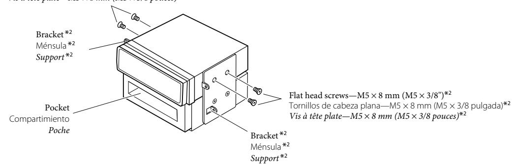
**Note** : When installing the unit on the mounting bracket, make sure to use the 8 mm (3/8") -long screws. If longer screws are used, they could damage the unit.
